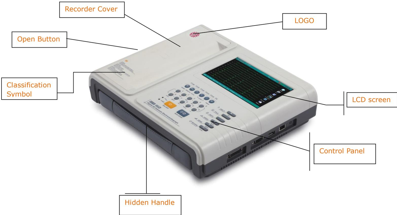
Figure 3-1 Front Panel of QRS-12
